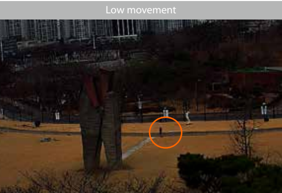
WiseStream II OFF : 7160kbps WiseStream II ON : 74kbps
